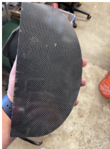
Fig 4: Cut carbon fiber ellipsoid fin prior to sanding
