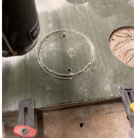
Fig 3: Bulkheads cut using X-Carve
