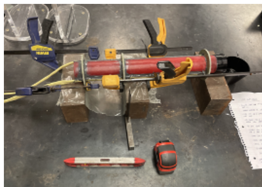
Fig 6: Epoxying front and middle centering rings
