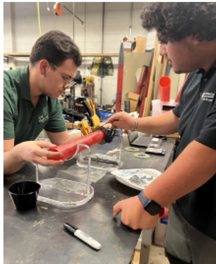
Fig 5: Epoxying rear centering ring
