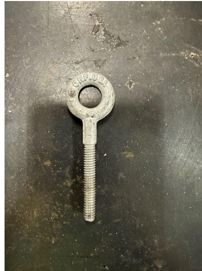
Fig 11: 1 of 3 eye bolts for avionics bay
