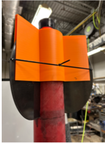
Fig 7: Orange fin guide used to keep fins 120 degrees apart
