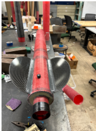
Fig 8: Fillets on booster tube and fins
