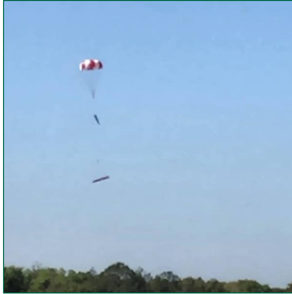
Figure 5: PDLs system after deployment during vehicle test flight.
