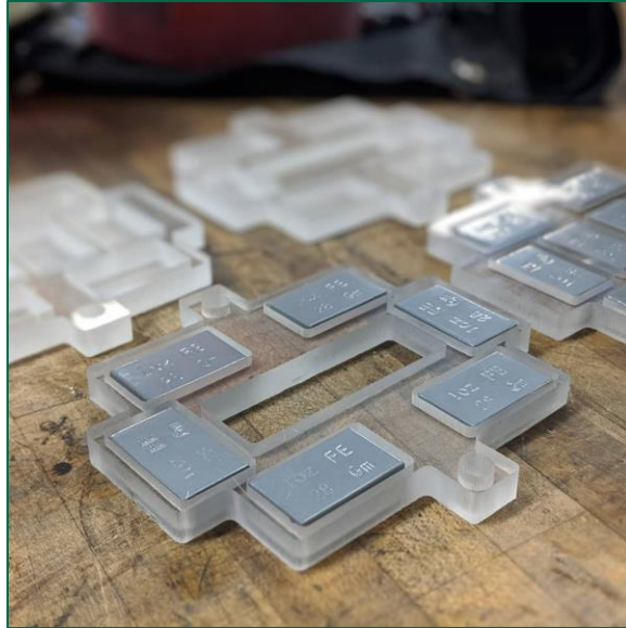
Figure 4: Constructed ABS plate with weights installed.
