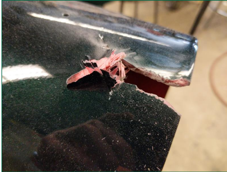
Figure 7: Damage to airframe due to PDLs failure, prior to repairs.
