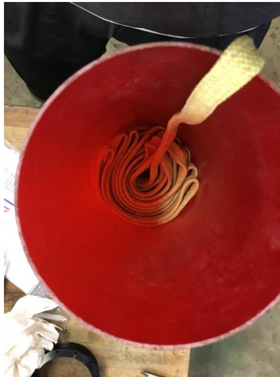
Figure 20: Layered Z-fold of shock cord inside airframe section.
