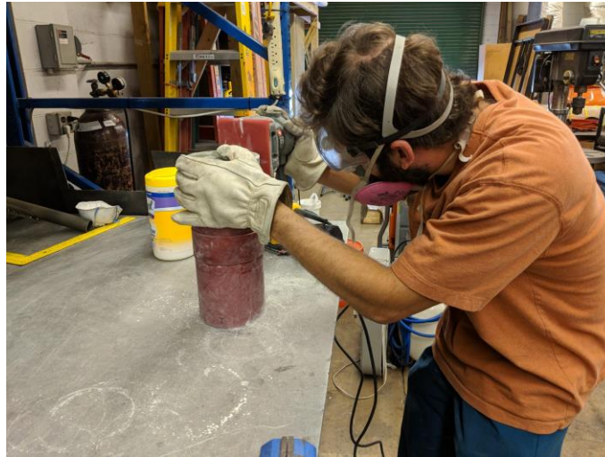
Figure 17: Sam works at sanding the fiberglass bulkheads to be flush with the G12 coupler.
