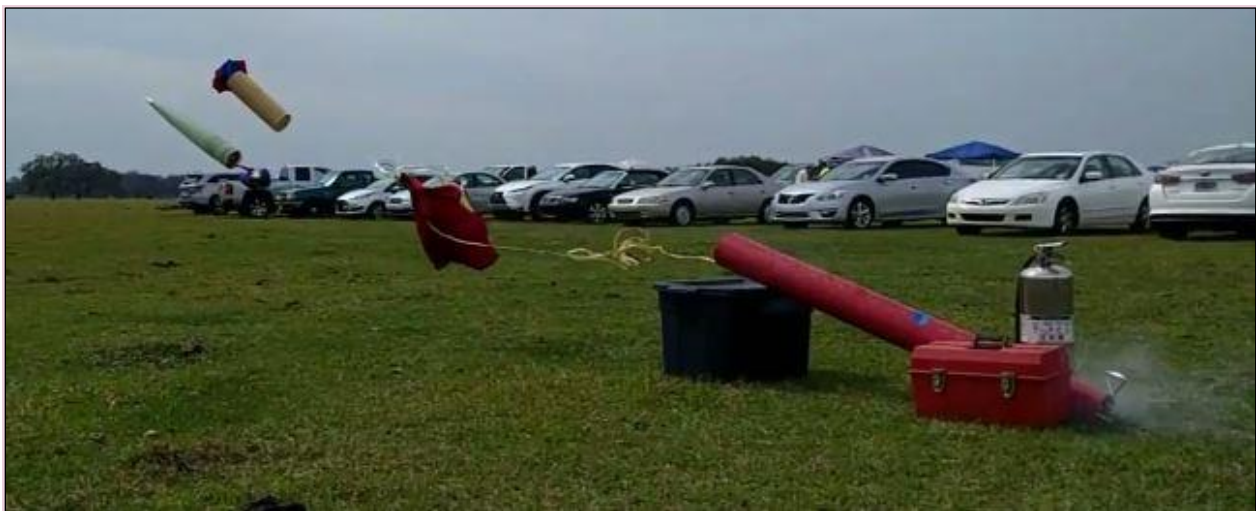
Figure 6: Successful full-scale recovery system ejection test.
