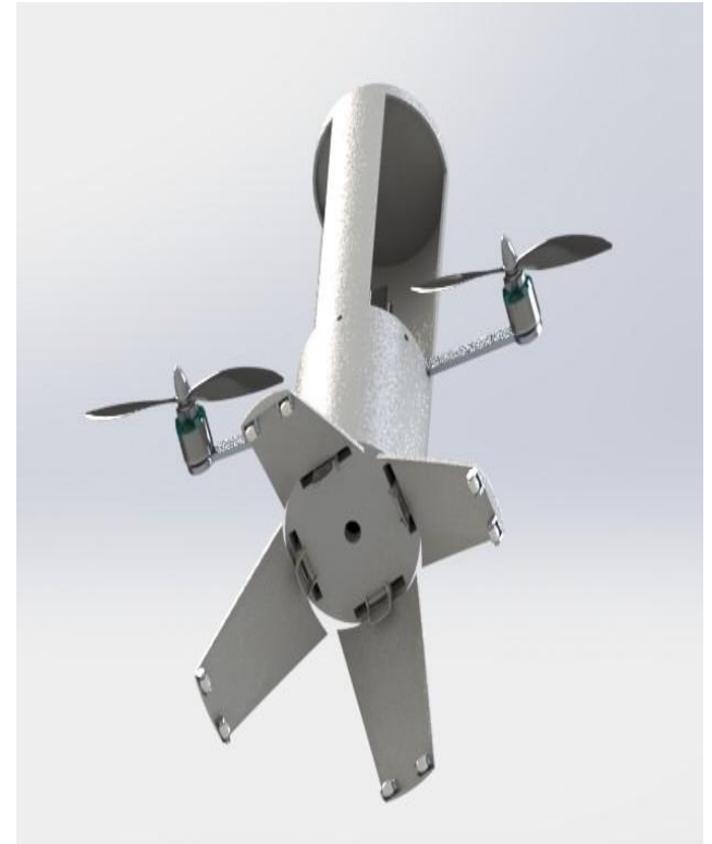
Figure 5: Landing Gear System Bottom View
