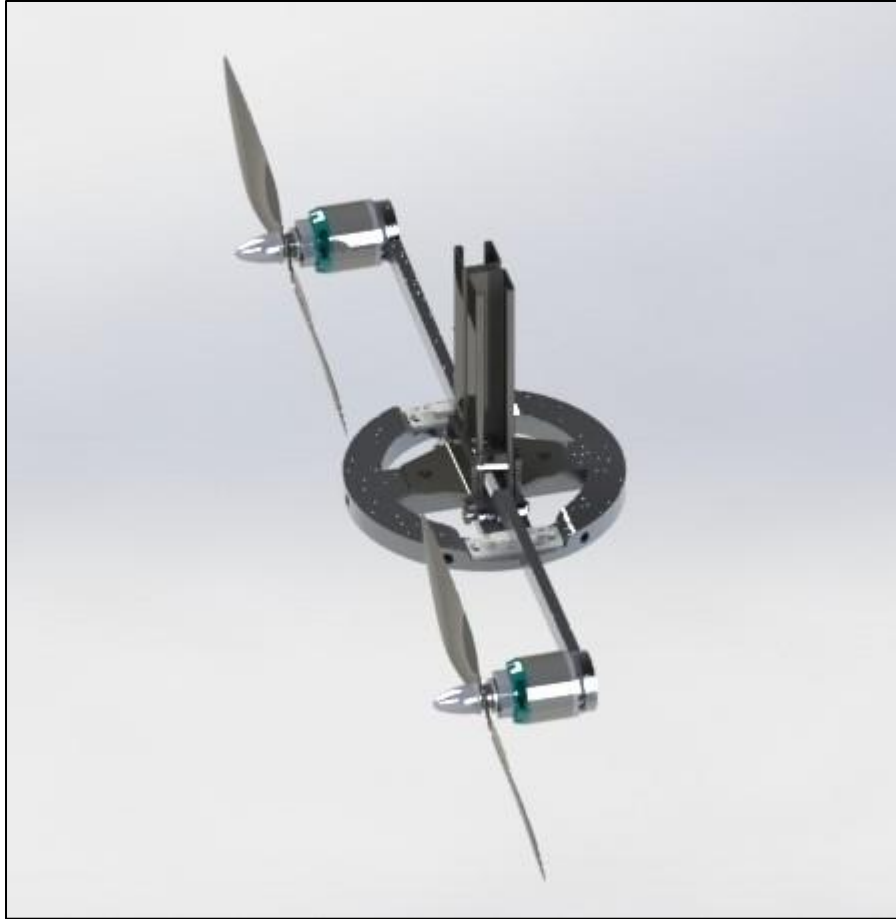
Figure 7 Isolated rendering of steering mechanism.
