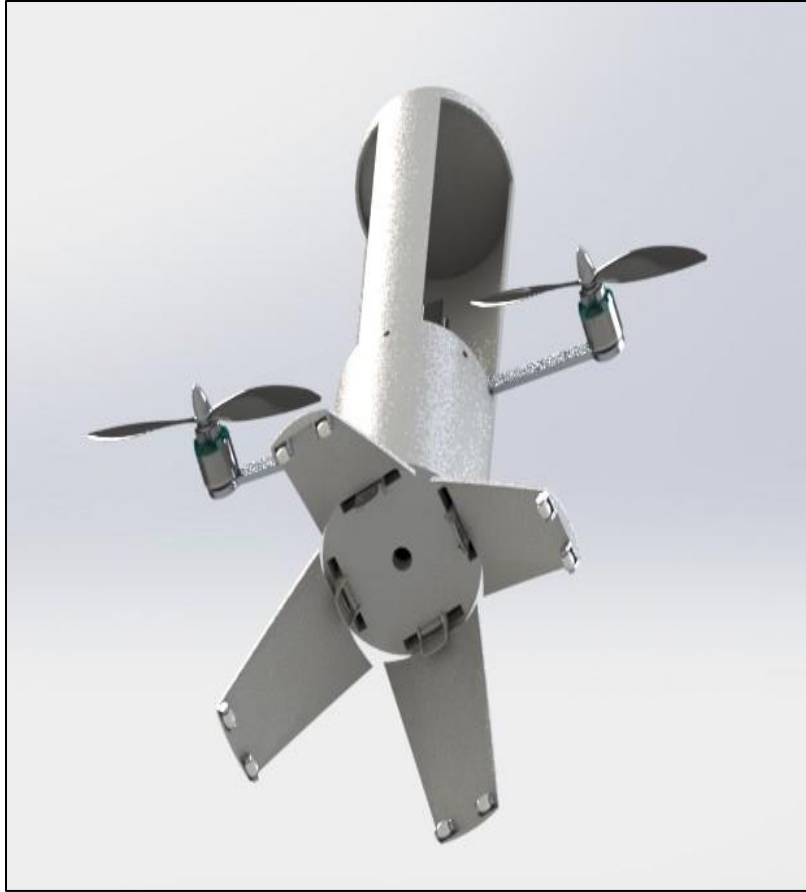
Figure 9: Rendering of the bottom of the landing gear system.
