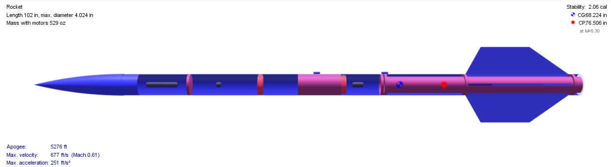
Figure 9: Launch Vehicle Model with CP as red dot (76.506 in) and CG as blue dot (68.224 in) as measured from the nose cone.
